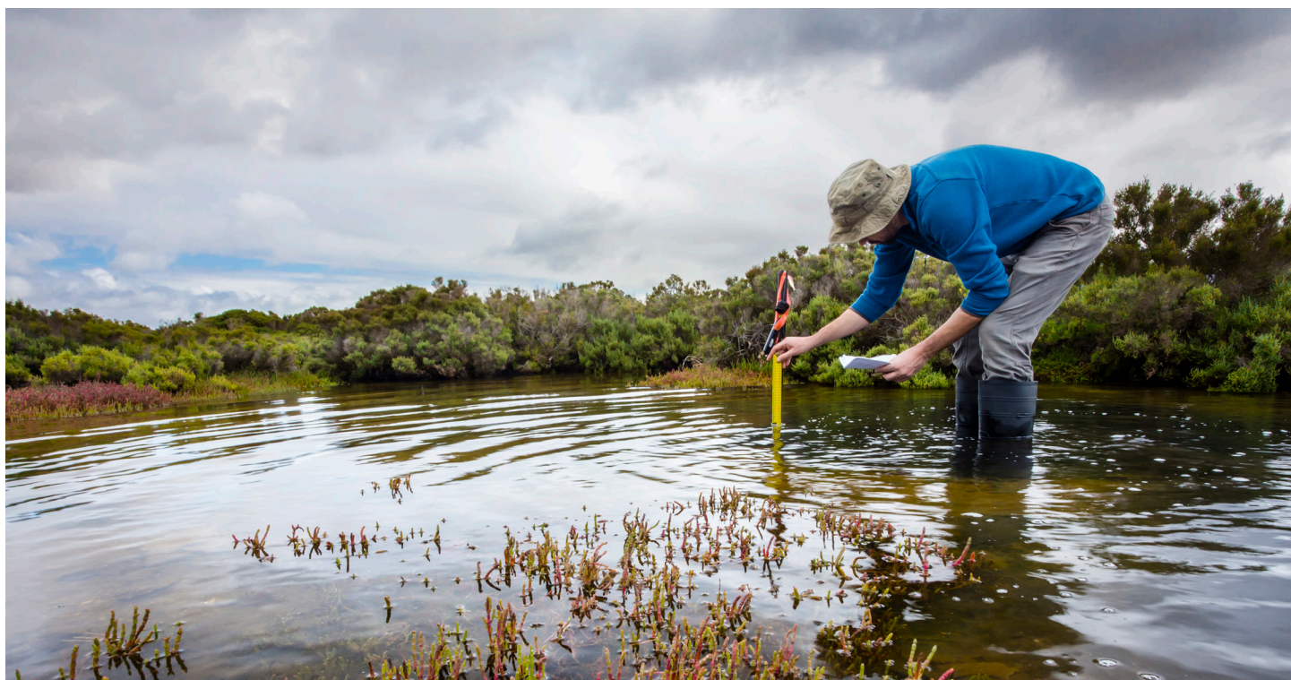
A scientist measures water depth in a coastal wetland before installing devices to record water level data. Getty Images/Tenedos
